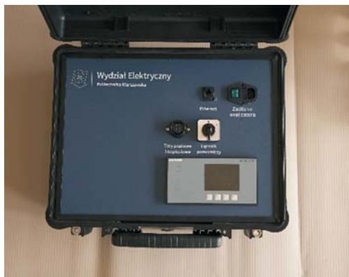
Wygląd walizki z analizatorem SICAM Q200 firmy Siemens | The appearance of the case with the Siemens SICAM Q200 analyzer
